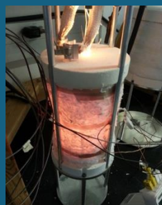
Heated sensor test rig at The Ohio State University Research Reactor, positioned near the core, for testing advanced sensors for nuclear reactors. (Prof. Raymond Cao, The Ohio State University)
