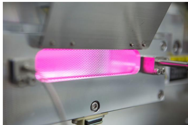
Figure 3 Glow of a processing plasma is seen through a port in the process chamber. The pink glow is due electrons exciting Argon atoms. (Source: TEL)
