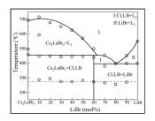
Crystal Growth and Optimization of Cs2LiLaBr6 Scintillator via the Cs2LaBr5-LiBr Phase Diagram Construction
