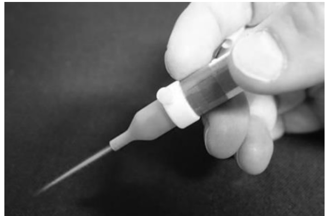
Fig. 4 Plasma jet driven by a piezoelectric transformer. Photo courtesy Dr. Claire Tendo
