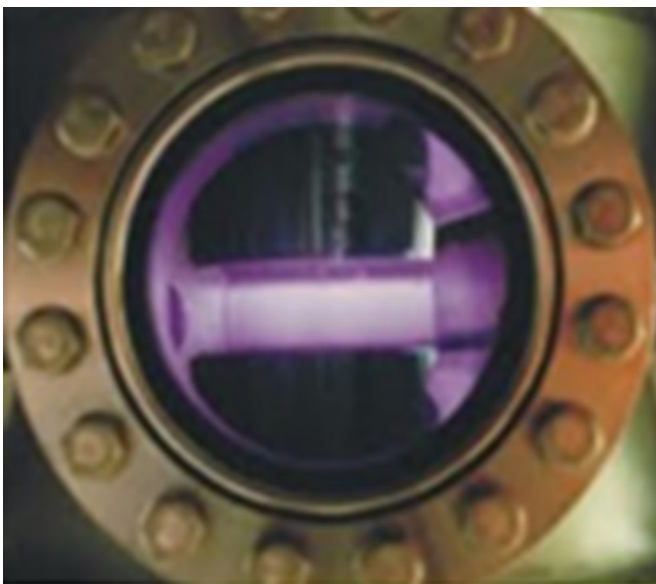
Fig. 1 Image of a low pressure plasma. The plasma is contained inside a vacuum chamber where working gas is introduced.
