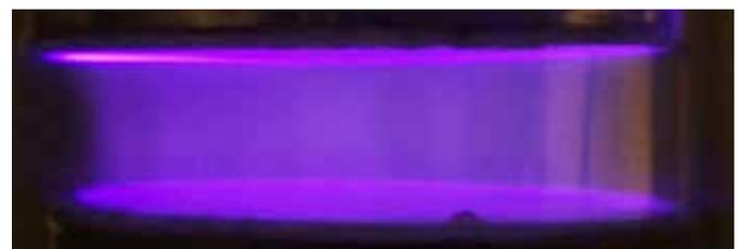
Fig. 1 Atmospheric pressure cold plasma generated by a dielectric barrier discharge. Photo courtesy M. Laroussi
