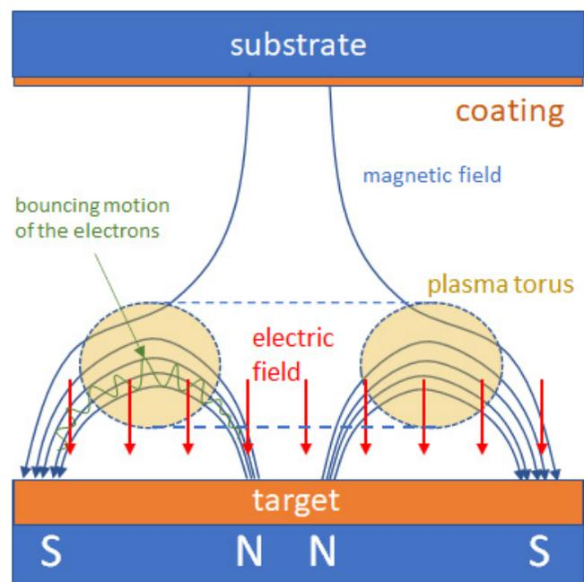
Fig. 1 Schematic of a magnetron plasma. The target (material to be sputtered) sits on a magnet and the substrate (material to be coated) faces the target.
