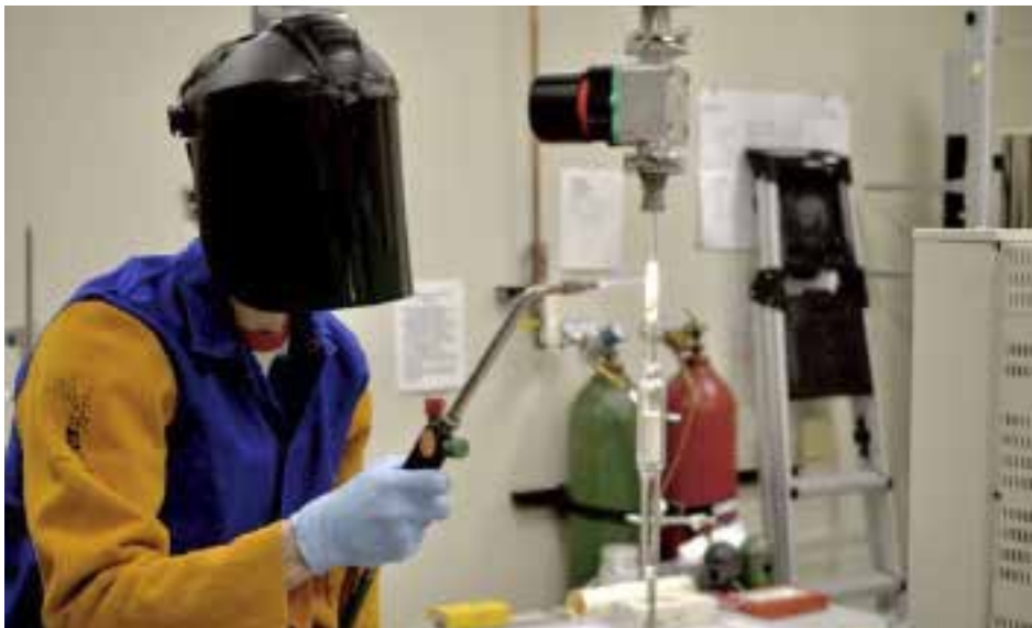
Fig. 1. Sealing an evacuated quartz ampoule loaded with raw material in preparation for crystal growth at the Scintillation Materials Research Center.
