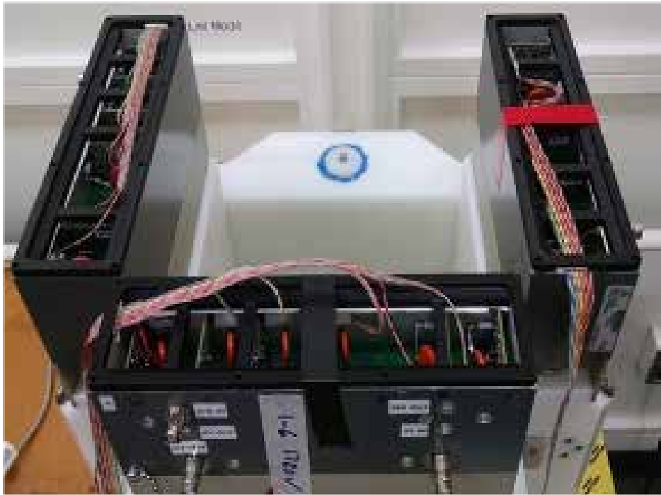
Fig. 5. New coincidence electronics designed for nondestructive assay instruments, here retrofitted to a Uranium Neutron Collar, for characterization with list mode data acquisition readout.
