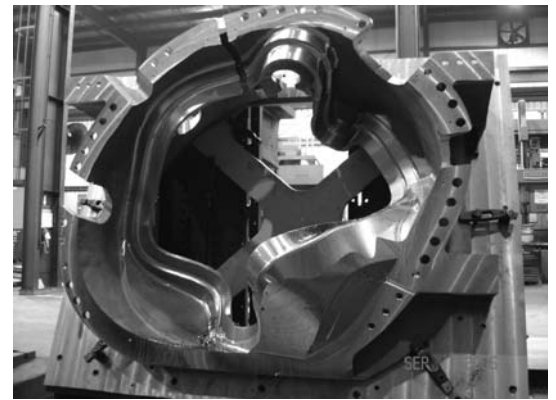
Fig. 3. Modular Coil Winding Form in manufacture.
