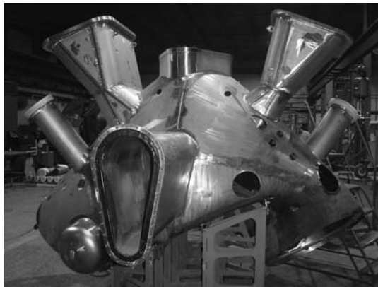
Fig. 2 Vacuum vessel segment in manufacture.
