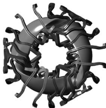
Fig. 1 NCSX plasma and modular coils.
